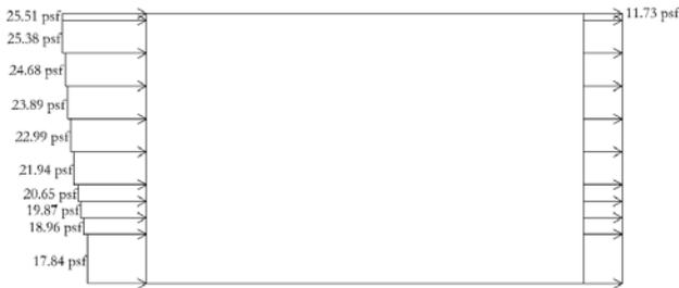
Figure 14: North-South Direction Wind Load
